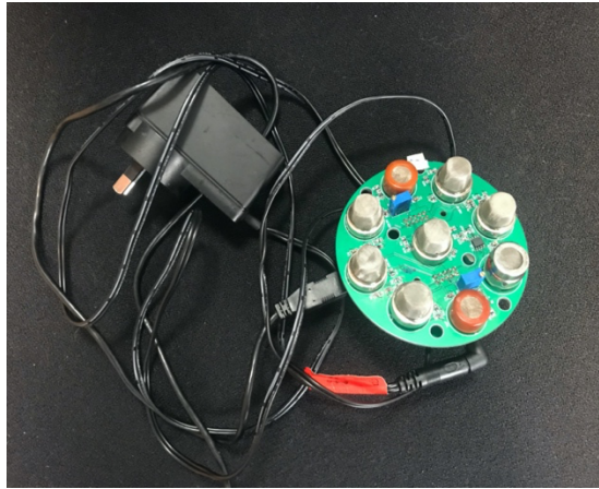
Figure 1. The front part of E-nose consists of nine sensors
