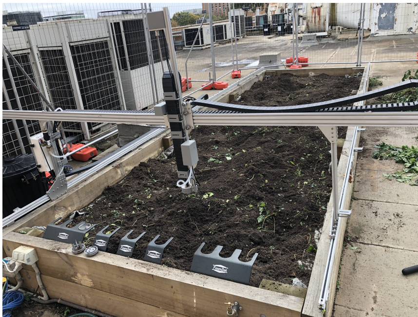
Fig. 1: Photo showing the simple design of the 3-axis Cartesian robot Farmbot
